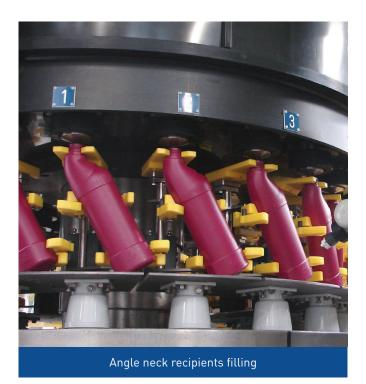
When designing its RC filling machine range, Serac has also emphasized flexibility by using the Plug-On<sup>®</sup> technology for format changes. Plug-on change tools enable the production of multiple formats on the same machine, with quick dismantling and assembling.
